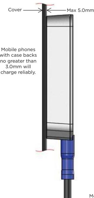
This is a module unit which must be installed within a further structure. Cover or structure over the coil area should not exceed 5.0 mm in thickness.
