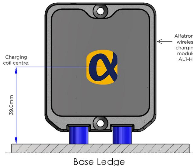
Most wireless mobile phones will connect within 5.0mm from optimal central point. If the installation includes a base ledge (on which the phone sits) this should ideally be placed 39.0mm from the centre of the AL1 series module for optimum performance with a wide variety of mobile phones.
